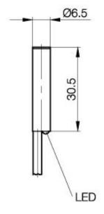
Inductive Sensors BES 516-372-G-E4-C-PU-05 D6.5 x 30.5 normally-open Sn=2mm shielded
